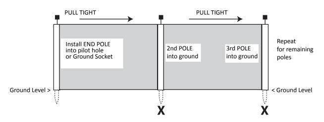
Installing single and multiple sets: Combine, configure and fit 150 and 50 ft. sets
